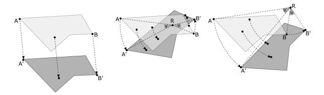
Please note: to perform a sliding motion in the corridor with the right-angled corner, all line segments (such as AA' and BB') must lie inside the corridor. For a rotation, all arcs (such as AA' en BB') must lie inside the corridor, but **point R does not necessarily have to lie inside the corridor**.
